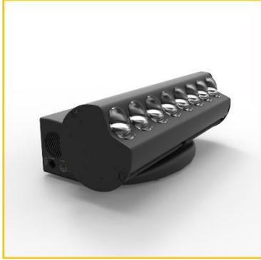
The new ADB KLEMANTIS is an asymmetric cyclight based on a six-colour LED module, which uses cutting-edge HCR (High Color Rendering) LED technology to deliver a wide selection of colors from bold hues to pastel shades. Thanks to an innovative algorithm, the unit is capable of achieving a stable CRI of over 97, as well as an impressive tunable white light ranging from 2500K to 8000K.
